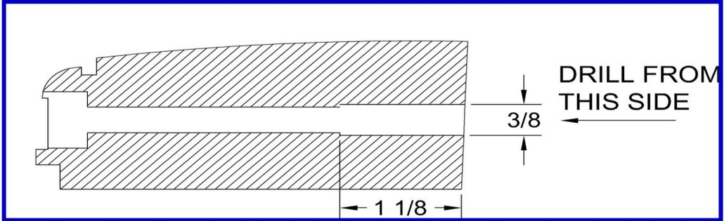
Drill the end mounting holes on the side rail using a 3/8" diameter drill bit. From the cushion side, drill no deeper than 1 1/8". This will allow just enough movement of the rail bolt so it can be angled to attach securely
