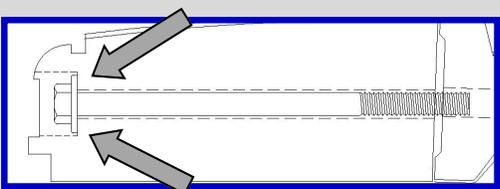
**WHAT IS THE PROPER CUSHION RAIL HEIGHT?** – BCA Specifications are 60% - 64% of the height of the object ball, or more simply measured: 1 7/16" above the bed of the table. Many people align the cushion rail even with the top rail laminate—usually putting the rails at or below the bottom-end of the specification. If you prefer to increase the speed or bounce of your rails, lower them at your own risk.
